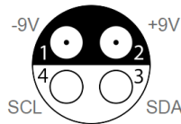
Probe’s power supply pin assignment “cable view”
